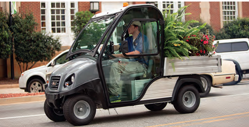
Club Car's Carryall electric, low speed vehicle has a total capacity of 1,250 pounds.
